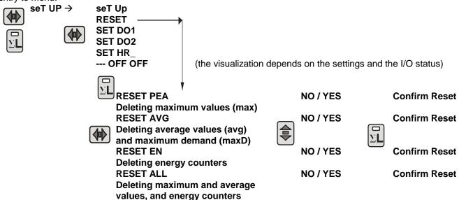
To enable the chosen type, press the **B** key to change the indication on display **G** from **NO** to **yes**. Confirm enabling cancellation, by pressing the **A** key. The indication on display **G** change from **yes** to --- .
