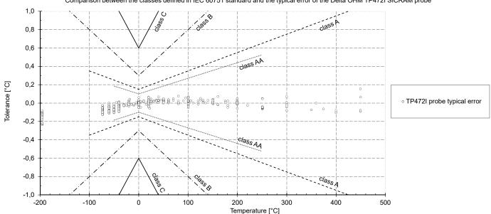
Comparison between the classes defined in IEC 60751 standard and the typical error of the Delta OHM TP472I SICRAM probe
