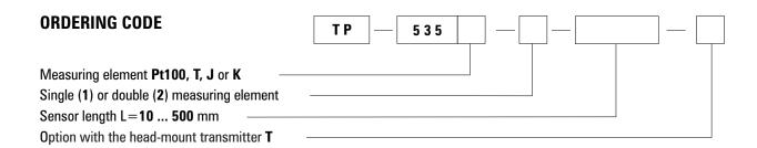
**Example for order:** TP-535Pt100-1-15 sensor with single Pt100 resistor of length L = 15 mm.
